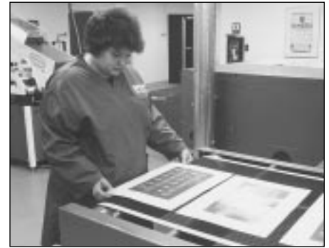
Figure 10. The curing/drying response of an ink can be evaluated with samples before major production work is started.
