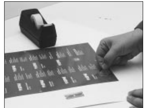
Figure 11. Testing the reaction and adhesion of an ink to a substrate can be accomplished with a sample ink deposit.
