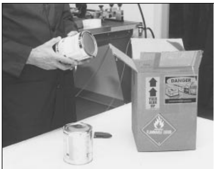
Figure 2. Incoming quality control can assure that only quality input is accepted and purchased for use in production. This is one reason why it is desirable to sample and test ink in a laboratory situation.
