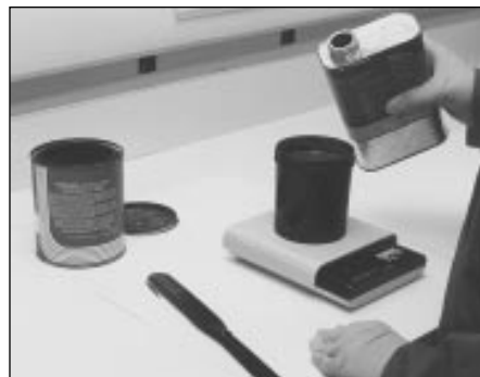
Figure 3. When modifying or combining ink it is important to test the resultant mixture to ensure its characteristics are within acceptable limits before introducing it into the production process.
